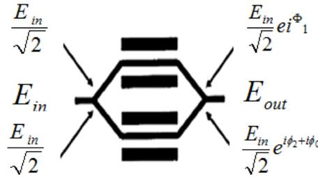
Figure 1.7 Electric field to MZM
